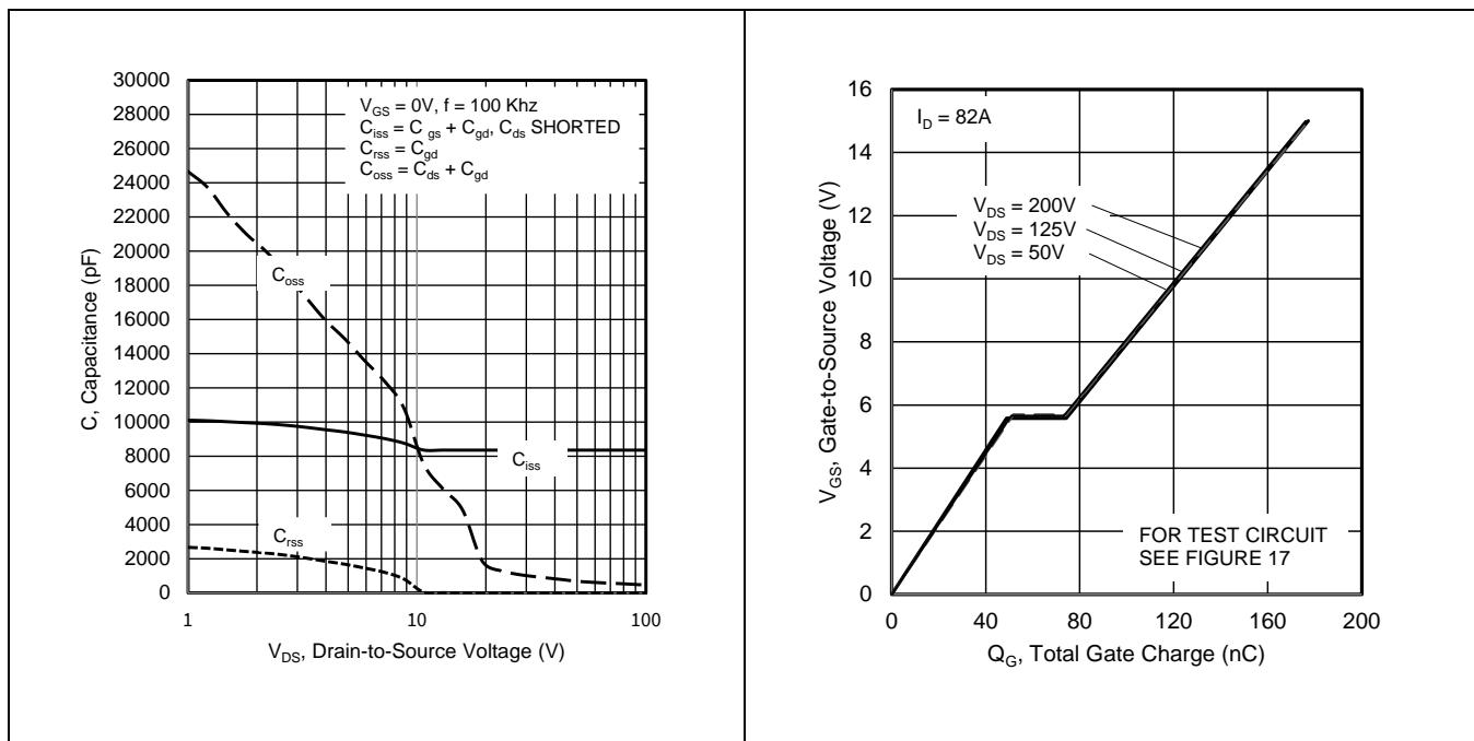
**Figure 10** Typical Capacitance Vs.
