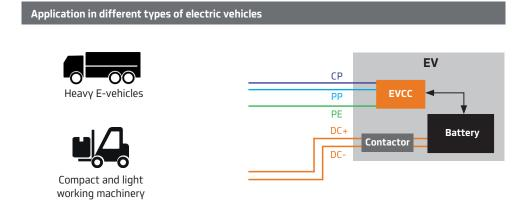
The DC Charging Controller is suitable for electric vehicles with high battery capacity. This includes the majority of the commercial vehicles. It can also be used in compact work vehicles with limited installation space.
