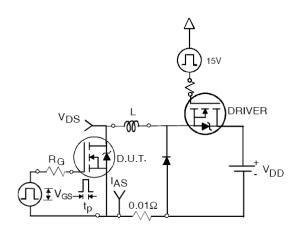
Fig 12a. Unclamped Inductive Test Circuit
