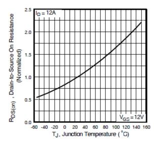
Fig 4. Normalized On-Resistance Vs. Temperature
