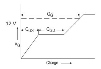
Fig 13a. Gate Charge Waveform
