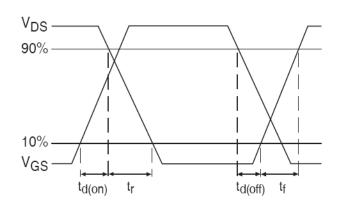
Fig 14b. Switching Time Waveforms
