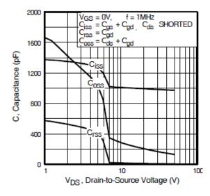
**Fig 5.** Typical Capacitance Vs. Drain-to-Source Voltage
