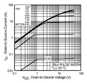
Fig 1. Typical Output Characteristics
