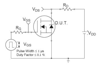
Fig 14a. Switching Time Test Circuit
