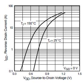
**Fig 7.** Typical Source-Drain Diode Forward Voltage
