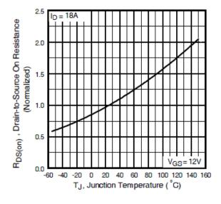
Fig 4. Normalized On-Resistance Vs. Temperature
