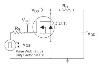
Fig 14a. Switching Time Test Circuit
