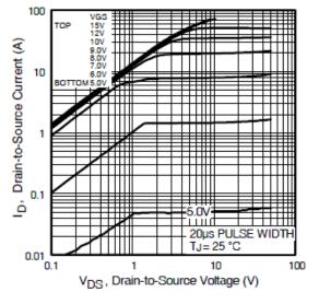
Fig 1. Typical Output Characteristics
