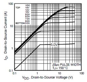
Fig 2. Typical Output Characteristics
