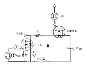
Fig 12a. Unclamped Inductive Test Circuit
