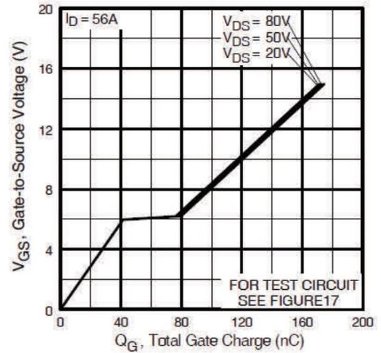
**Fig 10.** Typical Gate Charge Vs. Gate-to-Source Voltage
