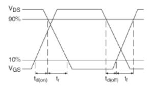
Fig 14b. Switching Time Waveforms
