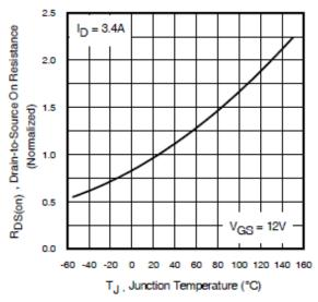
Fig 4. Normalized On-Resistance Vs. Temperature
