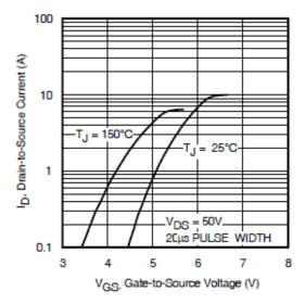
Fig 3. Typical Transfer Characteristics
