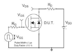
Fig 14a. Switching Time Test Circuit
