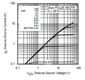
Fig 1. Typical Output Characteristics
