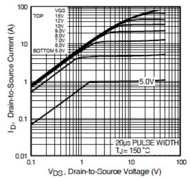
Fig 2. Typical Output Characteristics
