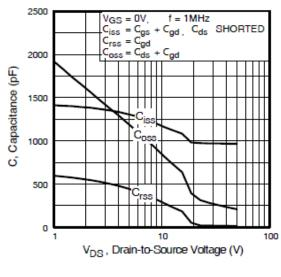
Fig 5. Typical Capacitance Vs. Drain-to-Source Voltage
