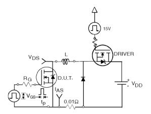
Fig 12a. Unclamped Inductive Test Circuit
