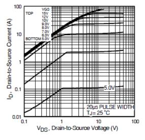
Fig 1. Typical Output Characteristics
