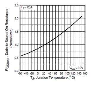
Fig 4. Normalized On-Resistance Vs. Temperature
