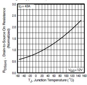
Fig 4. Normalized On-Resistance Vs. Temperature
