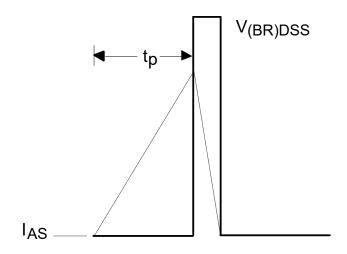
Fig 12b. Unclamped Inductive Wave-
