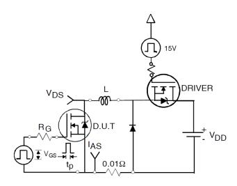
Fig 12a. Unclamped Inductive Test Circuit
