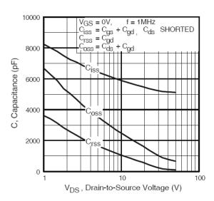
**Fig 5.** Typical Capacitance Vs. Drain-to-Source Voltage
