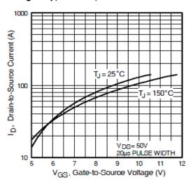
Fig 3. Typical Transfer Characteristics
