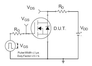
Fig 14a. Switching Time Test Circuit
