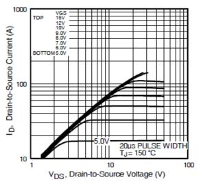
Fig 2. Typical Output Characteristics
