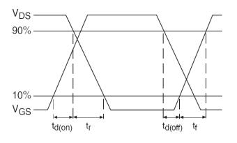
Fig 14b. Switching Time Waveforms
