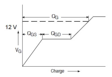
Fig 13a. Gate Charge Waveform
