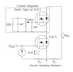
Fig 13b. Gate Charge Test Circuit
