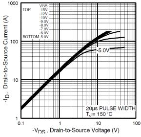
Fig 1. Typical Output Characteristics
