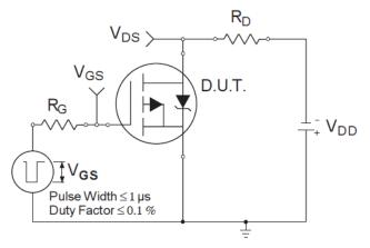
Fig 14a. Switching Time Test Circuit
