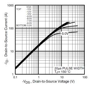
Fig 2. Typical Output Characteristics
