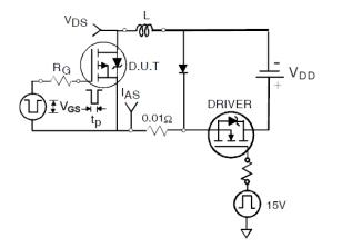
Fig 12a. Unclamped Inductive Test Circuit
