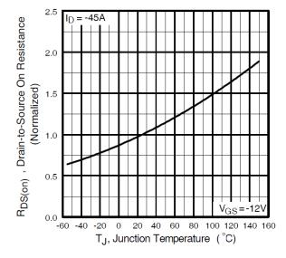
Fig 4. Normalized On-Resistance Vs. Temperature
