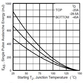
Fig 10. Maximum Avalanche Energy Vs. Drain Current
