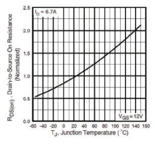
Fig 4. Normalized On-Resistance Vs. Temperature
