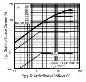
Fig 1. Typical Output Characteristics
