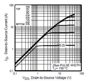
Fig 2. Typical Output Characteristics
