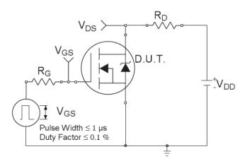
Fig 14a. Switching Time Test Circuit
