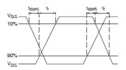
Fig 14b. Switching Time Waveforms
