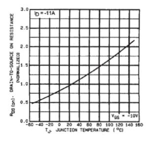
Fig 4. Normalized On-Resistance Vs. Temperature
