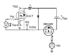
Fig 12a. Unclamped Inductive Test Circuit
