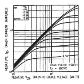
Fig 2. Typical Output Characteristics
