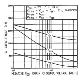
Fig 5. Typical Capacitance Vs. Drain-to-Source Voltage
