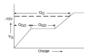
Fig 13a. Gate Charge Waveform
