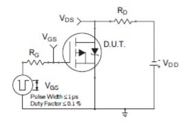
Fig 14a. Switching Time Test Circuit
