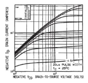
Fig 1. Typical Output Characteristics
