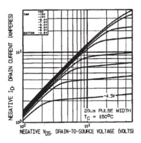
Fig 2. Typical Output Characteristics
