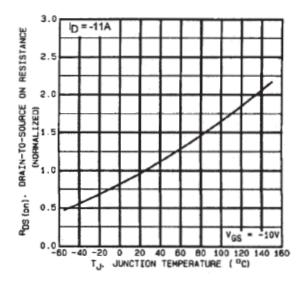
Fig 4. Normalized On-Resistance Vs. Temperature
