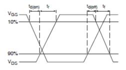
Fig 14b. Switching Time Waveforms
