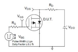
Fig 14a. Switching Time Test Circuit
