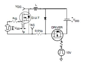
Fig 12a. Unclamped Inductive Test Circuit
