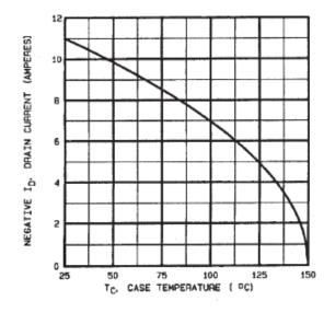
Fig 9. Maximum Drain Current Vs.Case Temperature
