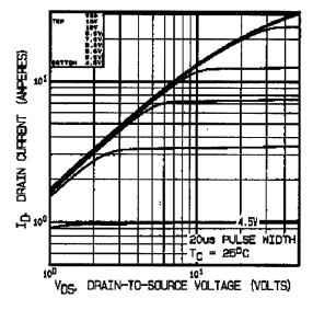
Fig 1. Typical Output Characteristics
