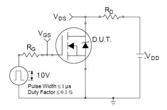
Fig 14a. Switching Time Test Circuit
