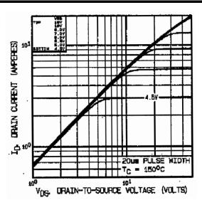
Fig 2. Typical Output Characteristics
