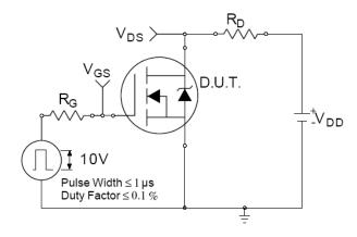
Fig 14a. Switching Time Test Circuit
