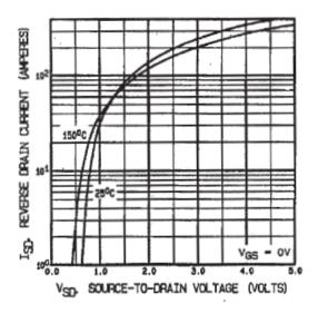
Fig 7. Typical Source-Drain Diode Forward Voltage
