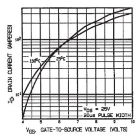
Fig 3. Typical Transfer Characteristics
