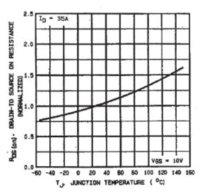
Fig 4. Normalized On-Resistance Vs. Temperature
