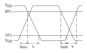
Fig 14b. Switching Time Waveforms
