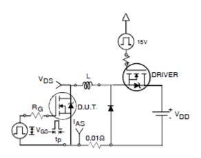
Fig 12a. Unclamped Inductive Test Circuit
