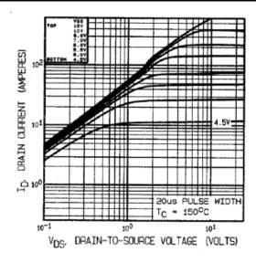
Fig 2. Typical Output Characteristics
