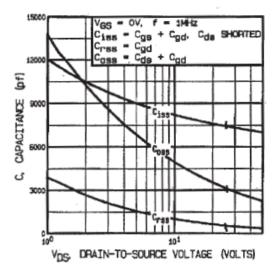
**Fig 5.** Typical Capacitance Vs. Drain-to-Source Voltage
