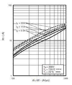
Fig. 6 Typical Recovery Current Vs di<sub>f</sub>/dt
