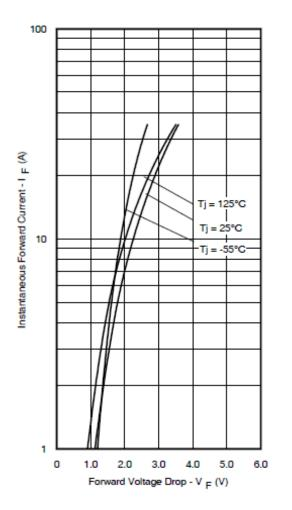
Fig. 1 Typical Forward Voltage Drop Vs. Instantaneous Forward Current
