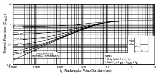
Fig. 4 Maximum Thermal Impedance Z<sub>thJC</sub> Characteristics
