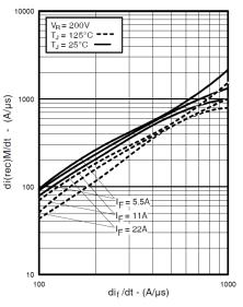
Fig. 8 Typical di<sub>(rec)M</sub>/dt Vs di<sub>f</sub>/dt
