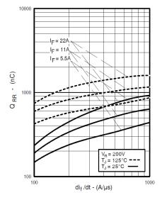
Fig. 7 Typical Stored Charge Vs  $di_f/dt$
