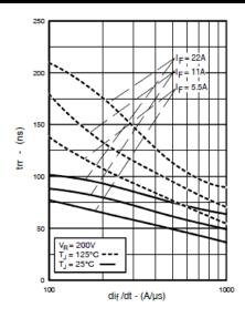
Fig. 5 Typical Reverse Recovery Vs di<sub>f</sub>/dt
