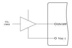
Figure 11. Direct Logic Drive
