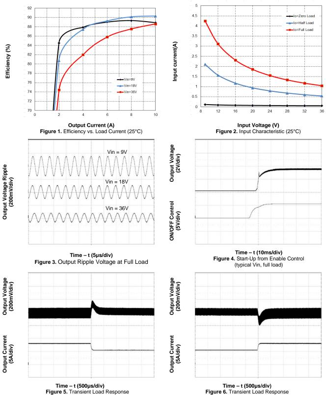
**Figure 5.** Transient Load Response (typical Vin, load current steps from 75% to 50% at a slew rate 0.1A/µs) **Time – t (500µs/div) Figure 6.** Transient Load Response (typical Vin, load current steps from 50% to 75% at a slew rate 0.1A/µs)
