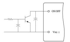
Figure 10. Open Collector Enable Circuit
