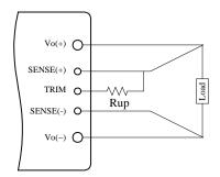
Figure 13. Circuit to Increase Output Voltage
