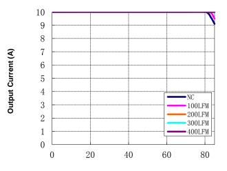
Ambient Temperature (°C) Figure 7. Current Derating Curve with Open Frame (Direction 3 (Ref. Figure 8); typical Vin, unit soldered onto a fixture board)
