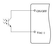
Figure 9. Opto Coupler Enable Circuit
