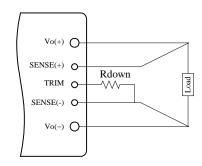
Figure 12. Circuit to Decrease Output Voltage
