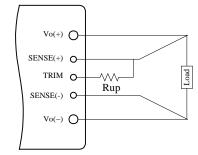
Figure 5. Circuit to Increase Output Voltage
