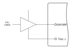
Figure 3. Direct Logic Drive
