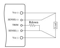
Figure 4. Circuit to Decrease Output Voltage
