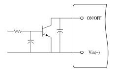
Figure 2. Open Collector Enable Circuit
