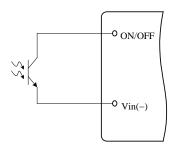
Figure 1. Opto Coupler Enable Circuit
