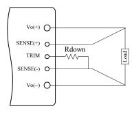
Figure 4. Circuit to Decrease Output Voltage
