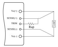
Figure 5. Circuit to Increase Output Voltage
