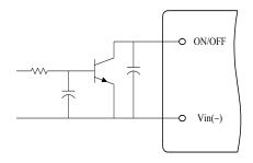
Figure 2. Open Collector Enable Circuit
