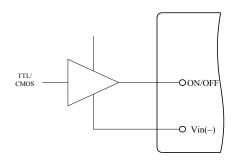
Figure 3. Direct Logic Drive
