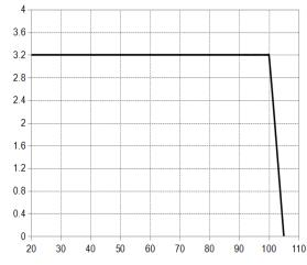
Baseplate Temperature (°C) QYR6A480x3A2xxx(x)-x (Vin=90V)
