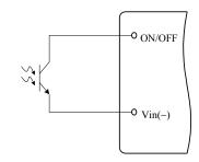
Figure 1. Opto Coupler Enable Circuit
