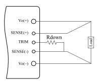
Figure 12. Circuit to Decrease Output Voltage
