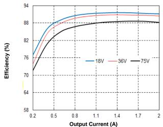
Figure 1. Efficiency vs. Load Current (25°C)
