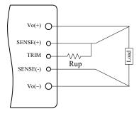
Figure 13. Circuit to Increase Output Voltage
