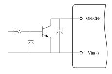
Figure 10. Open Collector Enable Circuit
