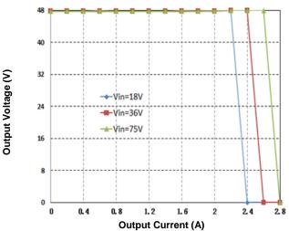
Figure 2. Output Characteristics (25°C)
