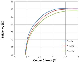
Figure 1. Efficiency vs. Load Current (25°C)
