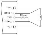
Figure 13. Circuit to Decrease Output Voltage
