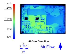
Figure 8. Thermal Image for Airflow Direction 3 (2A output, 55°C ambient, 200 LFM, typical Vin, open frame, unit soldered onto a fixture board)
