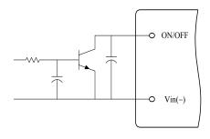
Figure 11. Open Collector Enable Circuit
