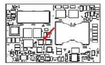
Figure 14. Temperature Monitoring Locations
