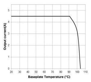
Figure 9. Derating Curve with baseplate temperature (typical Vin, baseplate unit soldered onto a fixture board)
