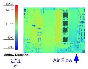
Figure 8. Thermal Image for Airflow Direction 1 (3A output, 55°C ambient 200 LFM, typical Vin, open frame, unit soldered onto a fixture board.)
