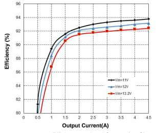
Figure 1. Efficiency vs. Load Current (25°C)
