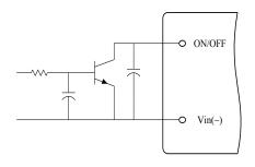
Figure 11. Open Collector Enable Circuit
