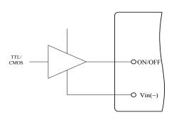
Figure 12. Direct Logic Drive
