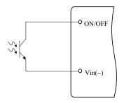
Figure 10. Opto Coupler Enable Circuit
