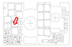
Figure 13. Temperature Monitoring Location
