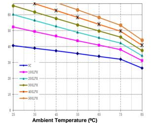
Figure 11. Derating Curve for Airflow Direction 3
