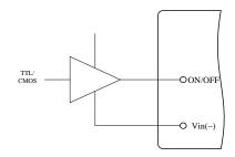
Figure 15. Direct Logic Drive
