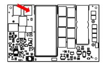
Figure 21. Temperature Monitoring Location
