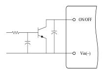
Figure 14. Open Collector Enable Circuit
