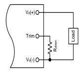
Figure 16. Circuit to Decrease Output Voltage Set Point
