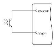
Figure 13. Opto Coupler Enable Circuit
