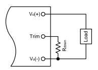
Figure 15. Circuit to Decrease Output Voltage
