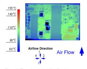
Figure 10. Thermal Image for Airflow Direction 3 (22.5A output, 55°C ambient, 200 LFM, typical Vin, open frame, soldered interface)
