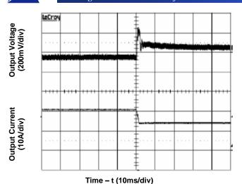
Figure 7. Transient Load Response
