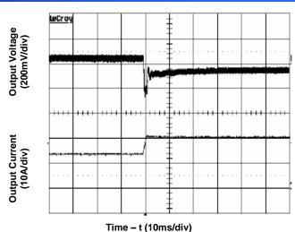
Figure 8. Transient Load Response (typical Vin, load current steps from 50% to 75% at a slew rate 0.1Α/μs)
