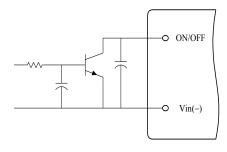
Figure 13. Open Collector Enable Circuit
