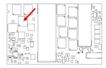
Figure 17. Temperature Monitoring Locations
