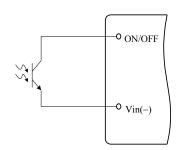
Figure 12. Opto Coupler Enable Circuit
