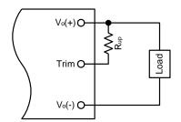
Figure 16. Circuit to Increase Output Voltage
