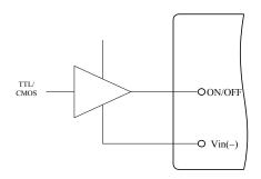
Figure 14. Direct Logic Drive
