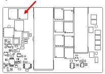
Figure 17. Temperature Monitoring Locations
