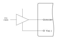
Figure 14. Direct Logic Drive
