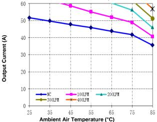
Figure 11. Current Derating Curve With Baseplate
