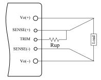
Figure 16. Circuit to Increase Output Voltage
