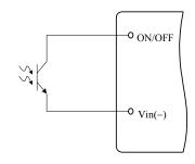
Figure 12. Opto Coupler Enable Circuit
