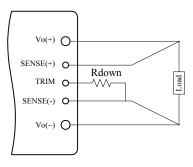
Figure 15. Circuit to Decrease Output Voltage
