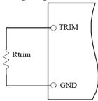
Figure 7. Circuit to Trim Output Voltage
