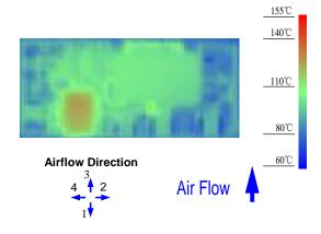
Figure 11. Thermal Image. Vin = 24V, 3.3V/6.5A output,  $55^{\circ}$  C ambient, 200 LFM
