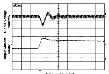
Time—t (50 $\mu$ s/div) Figure 9. Transient Load Response Vo = 3.3V, Vin = 24V, Io: 1.6A->3.5A,Slew rate 0.1A/ $\mu$ s.
