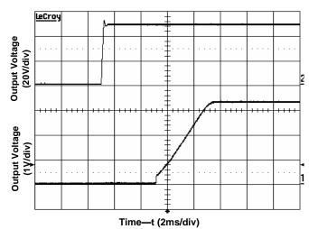
Figure 7. Start-Up from Application of Input Volatge Vin=24V, Vo=3.3V,lo=3.5A
