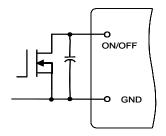
Fig. 13. Circuit for Positive Logic Control
