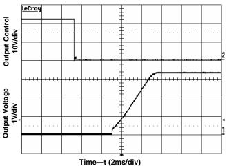
Figure 6. Start-Up from Enable Control Vin=24V, Vo=3.3V,lo=0A
