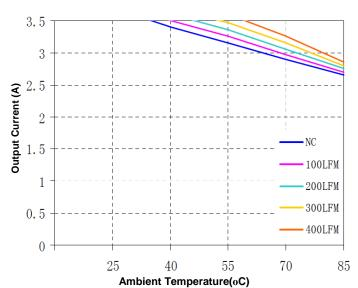
Figure 12(b) Current Derating Curve for Vo=5.0V and Vin=24V
