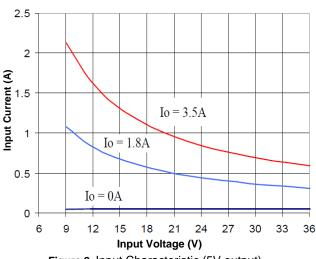
Figure 2. Input Characteristic (5V output)
