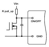
Fig. 14. Circuit for Negative Logic Control
