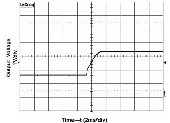
Figure 3. Start-Up with Prebias Vin = 24V, Vo= 3.3V, Io = 0A, Prebias 1.8V
