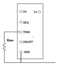
Figure 15. Circuit to Trim Output Voltage
