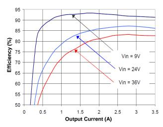
Figure 1(b). Efficiency vs. Load Current (25°C, 5.0V)
