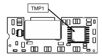
**Figure 16.** NBS Bottom View — Temperature Monitoring Point TMP1 for Thermal Shutdown
