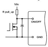
Fig. 14. Circuit for Negative Logic Control
