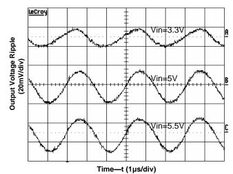
Figure 4. Output Ripple Voltage at 1=2.5V, 8A Output
