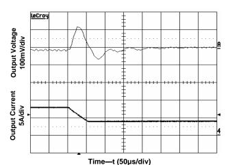
Figure 7. Transient Load Response Input voltage 5V, Output current 4A(50% full load), Slew rate 0.2A/µs.
