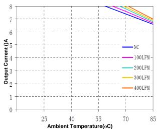
Figure 13(c) Current Derating Curve for 1.0V Output (Vin = 5V open frame)
