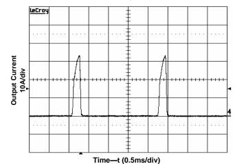
Figure 10. Short Circuit Current. Vin = 5V
