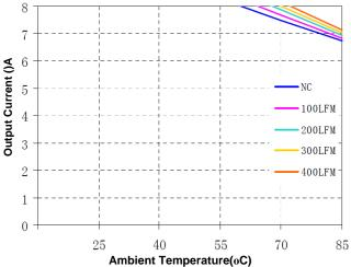
Figure 12(e) Current Derating Curve for 2.5V Output
