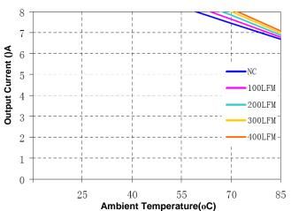
Figure 13(d) Current Derating Curve for 1.8V Output
