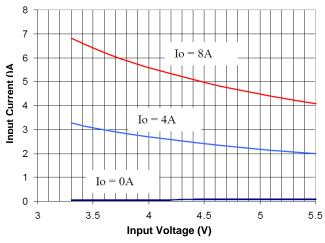
Figure 2. Input Characteristic (2.5V output)
