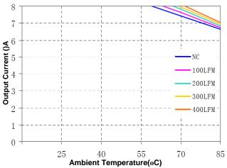
Figure 13(c) Current Derating Curve for 1.5V Output (Vin = 5Vopen frame)
