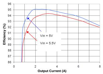
Figure 1(d). Efficiency vs. Load Current (25°C, 3.3V)
