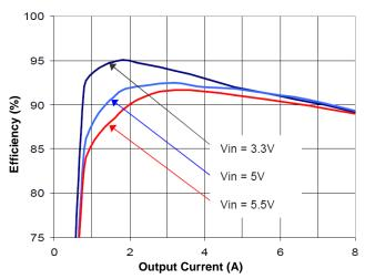
Figure 1(b). Efficiency vs. Load Current (25°C, 2.5V)
