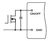
Fig. 13. Circuit for Positive Logic Control
