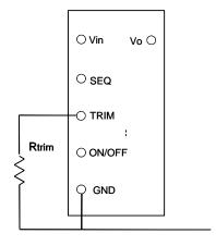
Fig. 15. Circuit to Trim Output Voltage
