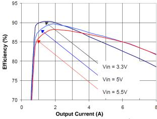
Figure 1(c). Efficiency vs. Load Current (25°C, 1.2V)
