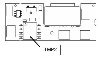
Figure 17. NBS Top View — Temperature Monitoring
