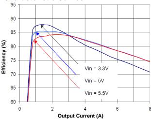
Figure 1(a). Efficiency vs. Load Current (25°C, 0.75V)
