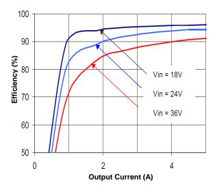
Figure 1(b). Efficiency vs. Load Current (25°C, 12V)
