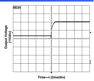
Figure 3.Start-Up with Prebias (25°C, 5V) (Input voltage 24V, Output current 0A, Output voltage 5V, Prebias 3.3V)
