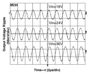
Figure 7.Output Reflected Ripple at 12V, 5A Output
