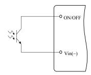
Figure 12. Circuit for Positive Logic Control
