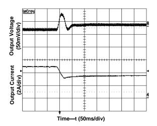
Figure 8.Transient Load Response (Input/output voltage 24/12V, Output current 5A->3.75A, Slew rate 0.1A/µs)
