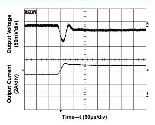
Figure 9.Transient Load Response (Input voltage 24/12V, Output current 3.75A->5A, Slew rate 0.1A/µs)
