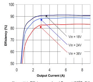
Figure 1(a). Efficiency vs. Load Current (25°C, 5V)
