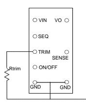
Figure 14. Circuit to Trim Output Voltage
