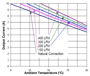
Figure 11.Current Derating Curve for 5V Output (Vin = 12V open frame)
