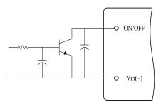
Figure 13. Circuit for Negative Logic Control
