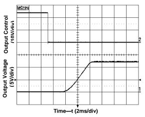
Figure 4.Start-Up from Enable Control (Input voltage 24V, Output current 5A 12V)
