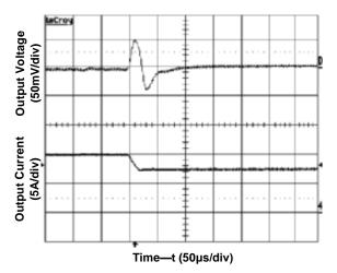
Figure 8. Transient Load Response Input/output voltage 24/3.3V,Output current 10A->7.5A,Slew rate 0.1A/μs
