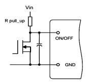
Figure 13. Circuit for Logic Control
