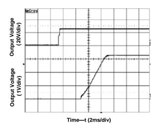
Figure 5. Start-Up from Application of Input Voltage (Input voltage 24V, Output current 10A 3.3V)
