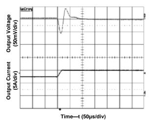
Figure 9. Transient Load Response Input voltage 24/3.3V, Output current 7.5A->10A, Slew rate 0.1A/µs
