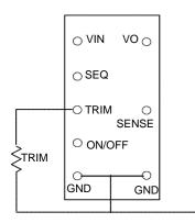
Figure 14. Circuit to Trim Output Voltage.
