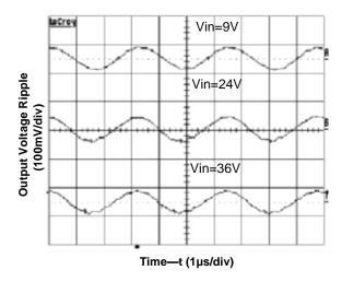
Figure 7. Output Reflected Ripple at 3.3V, 10A Output
