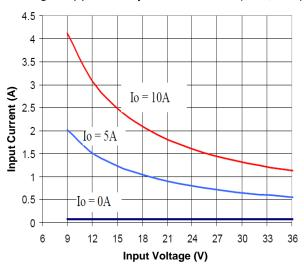
Figure 2. Input Characteristic (5V output)
