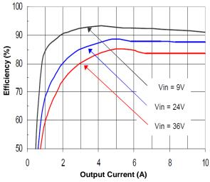
Figure 1(a). Efficiency vs. Load Current (25°C, 3.3V)
