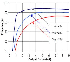
Figure 1(b). Efficiency vs. Load Current (25°C, 5V)
