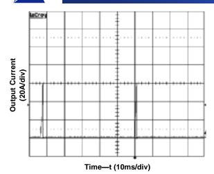
Figure 10. Short Circuit Current. Vin = 24
