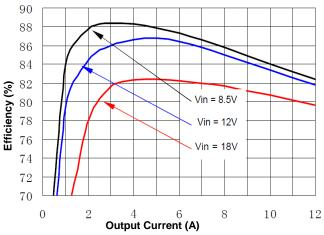
Figure 1(c). Efficiency vs. Load Current (25°C, 1.2V)
