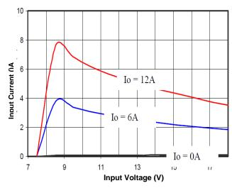
Figure 7 Input Characteristic (5V output)
