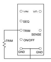
Fig. 15 Circuit to Trim Output Voltage.
