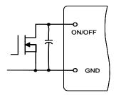
Fig. 13 Circuit for Positive Logic Control
