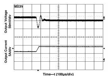
Figure 9 Transient Load Response
