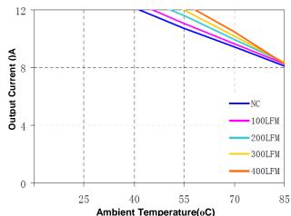
Figure 12(f) Current Derating Curve for 5.0V Output
