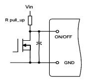
Fig. 14 Circuit for Negative Logic Control
