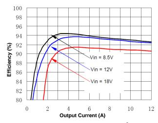
Figure 1(h). Efficiency vs. Load Current (25°C, 5V)
