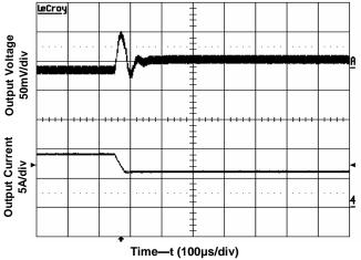
Figure 8 Transient Load Response Input voltage 12V, Output current 6A(50% full load), Slew rate 0.1A/µs.
