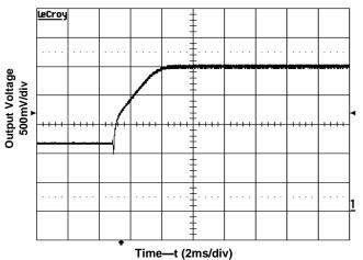
Figure 6. Start-Up with Prebias Input voltage 12V, Output current 0A, Output voltage 2.5V, Prebias 1.8V
