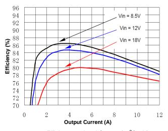
Figure 1(b). Efficiency vs. Load Current (25°C, 1V)
