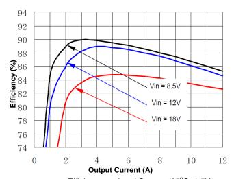
Figure 1(d). Efficiency vs. Load Current (25°C, 1.5V)
