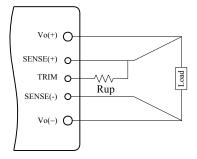
Figure 16. Circuit to Increase Output Voltage
