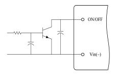
Figure 13. Open Collector Enable Circuit
