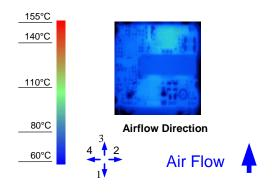
Figure 10. Thermal Image for Airflow Direction 3 (10A output, 55°C ambient, 200 LFM, typical Vin, open frame unit)
