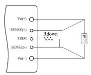
Figure 15. Circuit to Decrease Output Voltage
