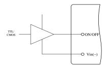
Figure 14. Direct Logic Drive
