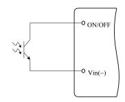
Figure 12. Opto Coupler Enable Circuit
