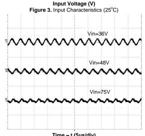
Output Voltage Ripple (100mV/div)
