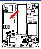
Figure 17. Temperature Monitoring Locations
