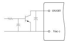
Figure 2. Open Collector Enable Circuit
