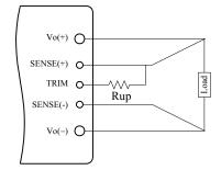
Figure 5. Circuit to Increase Output Voltage
