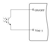
Figure 1. Opto Coupler Enable Circuit
