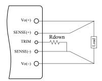
Figure 4. Circuit to Decrease Output Voltage
