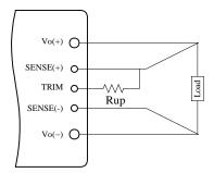
Figure 14. Circuit to Increase Output Voltage
