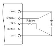
Figure 13. Circuit to Decrease Output Voltage
