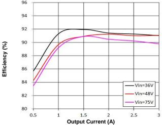
Figure 1. Efficiency vs. Load Current (25°C)
