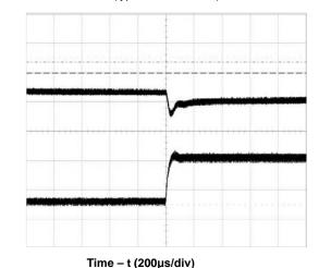
Figure 6. Transient Load Response (typical Vin, load current steps from 50% to 75% at a slew rate 0.1A/µs)
