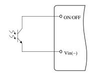
Figure 11. Opto Coupler Enable Circuit
