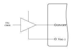
Figure 13. Direct Logic Drive
