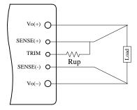
Figure 15. Circuit to Increase Output Voltage
