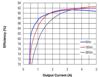
Figure 1. Efficiency vs. Load Current (25°C)
