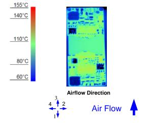
Figure 10. Thermal Image for Airflow Direction 3 (5A output, 55°C ambient, 200 LFM, typical Vin, open frame, unit soldered onto a fixture board)
