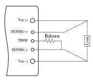
Figure 14. Circuit to Decrease Output Voltage
