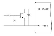
Figure 12. Open Collector Enable Circuit
