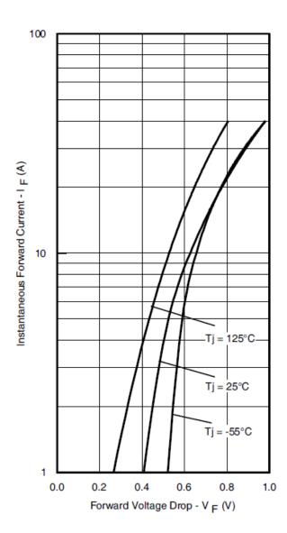
Fig 1. Max. Forward Voltage Drop Characteristics (Per Leg)
