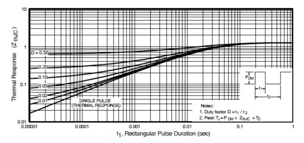
Fig 4. Max. Thermal Impedance ZthJC Characteristics (Per Leg)
