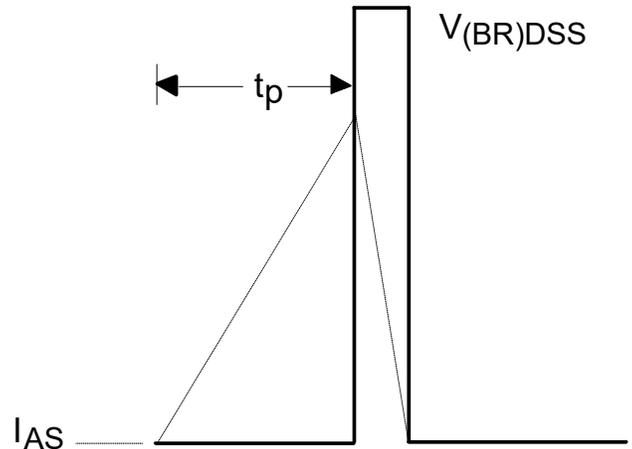
**Fig 12b.** Unclamped Inductive Wave-
