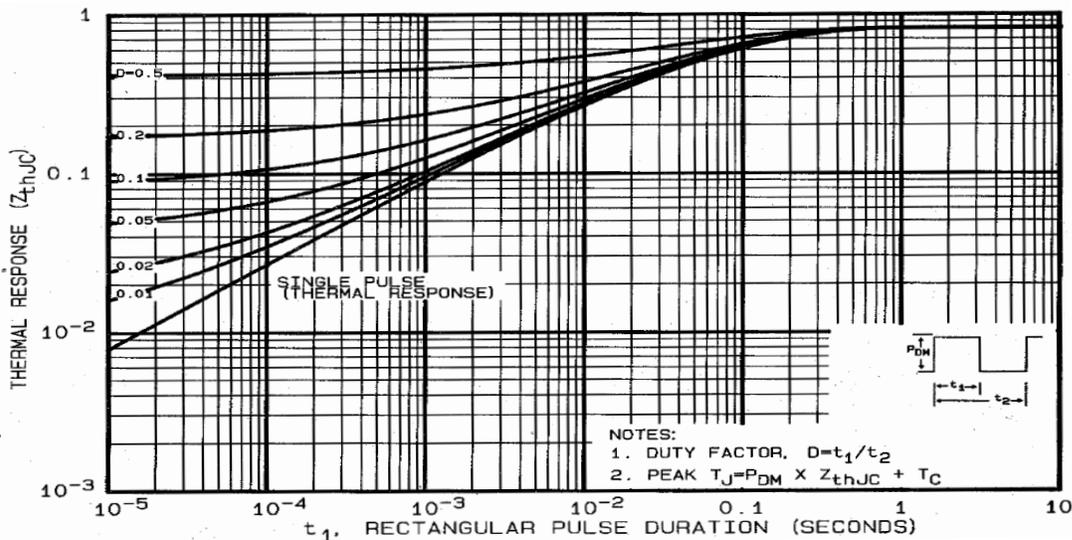
**Fig 11.** Maximum Effective Transient Thermal Impedance, Junction-to-Case
