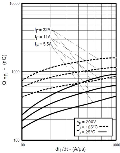
**Fig. 7** Typical Stored Charge Vs  $di_f/dt$
