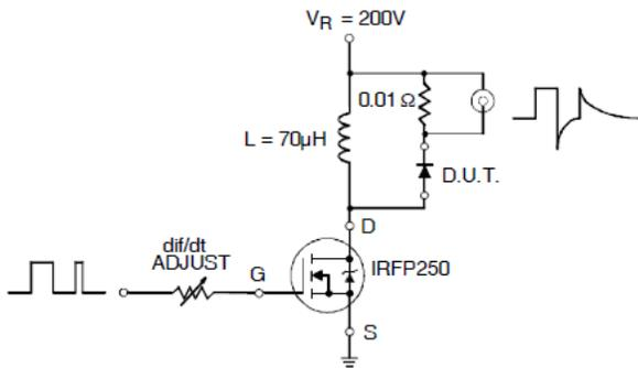
**Fig. 9** Typical Reverse Recovery Parameter Test Cir-
