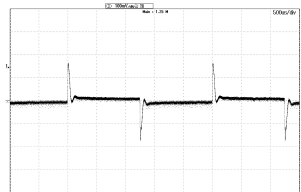
Figure 6: Step load 50%-100%, 100 mV/div and 500 us/div.
