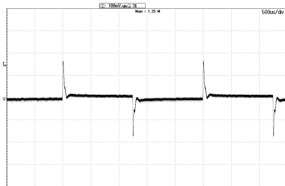
Figure 5: Step load 10%-50%, 100 mV/div and 500 us/div.
