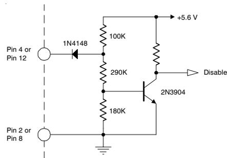
Internally, these ports differ slightly in their function. In use, a low on Enable 1 completely shuts down all circuits in the converter while a low on Enable 2 shuts down the secondary side while altering the controller duty cycle to near zero. Enabling by the use of either port is transparent to the user save for minor differences in idle current. (See specification table).
