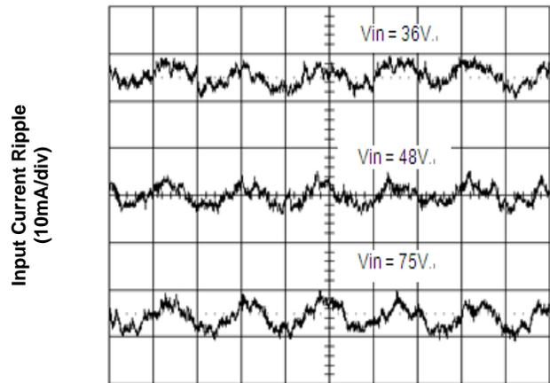
Figure 4. Input Reflected Ripple Current at Full Load
