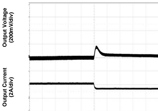
Figure 5. Transient Load Response (typical Vin, load current steps from 75% to 50% at a slew rate 0.1A/µs)
