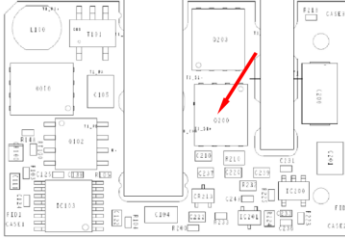
Figure 15. Temperature Monitoring Locations
