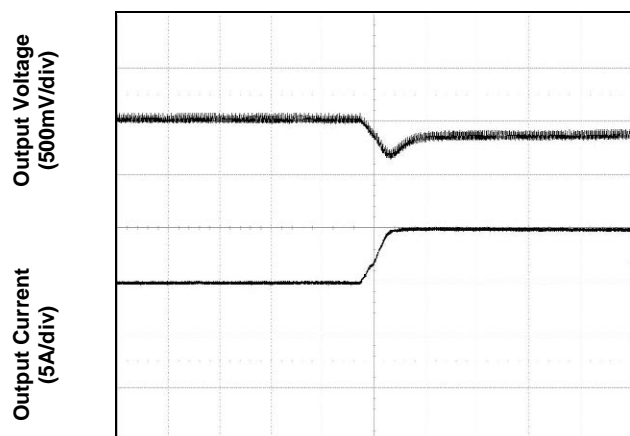
Figure 6. Transient Load Response (typical Vin, load current steps from 50% to 75% at a slew rate 0.1A/µs)
