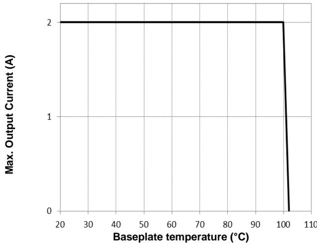
**Figure 9.** Current Derating Curve for Baseplate
