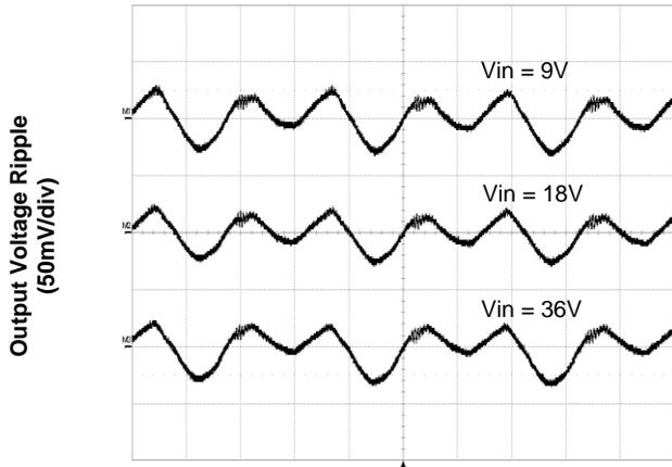
Figure 3. Output Ripple Voltage at Full Load
