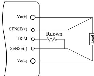
**Figure 13.** Circuit to Decrease Output Voltage
