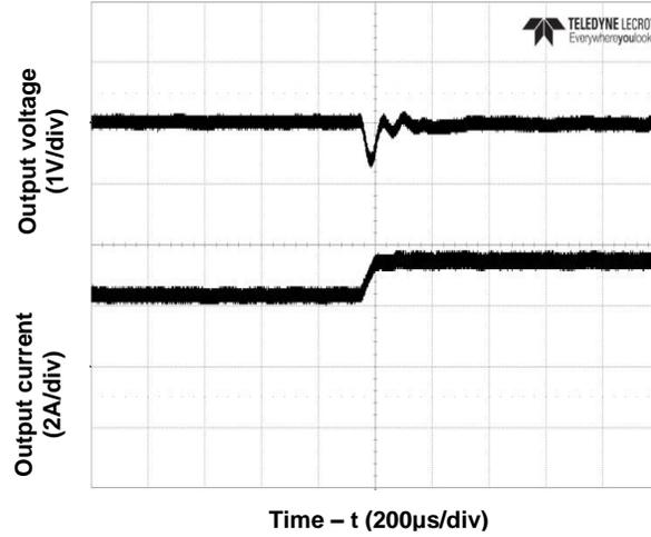
Figure 6. Transient Load Response
