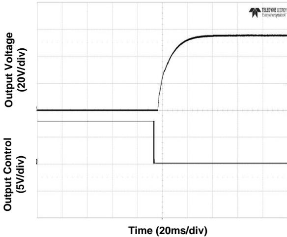
Figure 3. Start-Up from Enable Control
