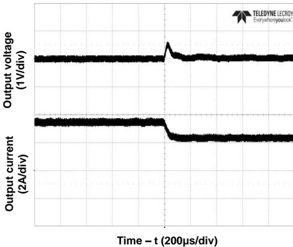
Figure 5. Transient Load Response
