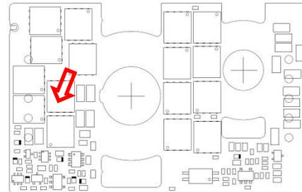
Figure 13. Temperature Monitoring Location
