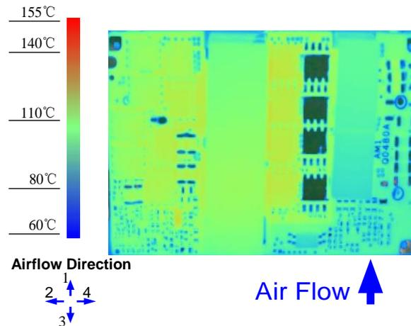
Figure 8. Thermal Image for Airflow Direction 1
