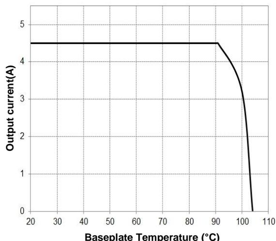
**Figure 9.** Derating Curve with baseplate temperature (typical  $V_{in}$ , baseplate unit soldered onto a fixture board)
