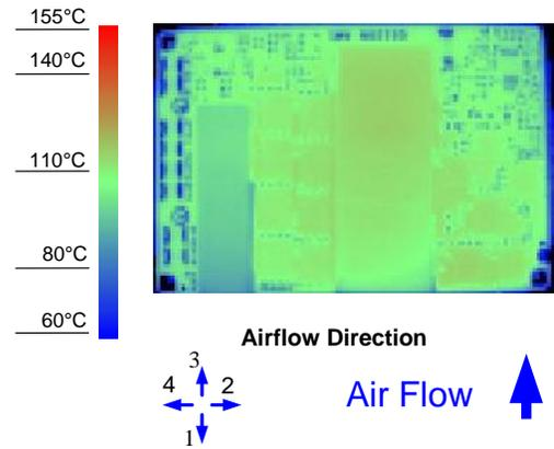
**Figure 10. Thermal Image for Airflow Direction 3**
