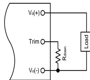
Figure 16. Circuit to Decrease Output Voltage Set Point
