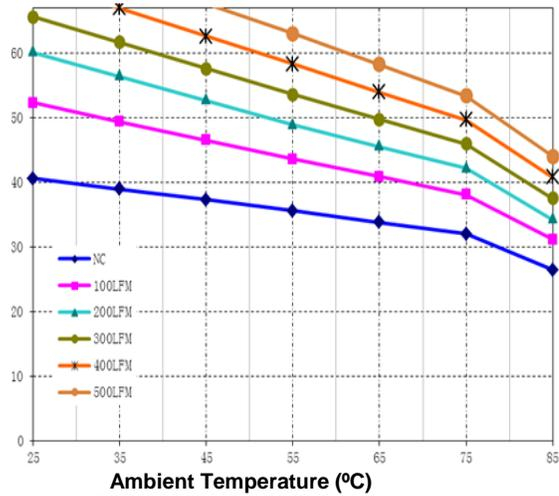
**Figure 12. Derating Curve for Airflow Direction 3**
