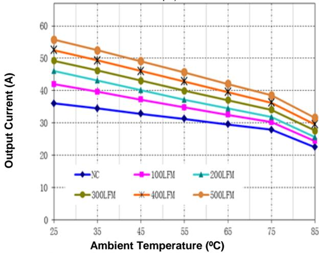
**Figure 9. Derating Curve for Airflow Direction 3**
