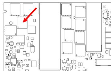
Figure 17. Temperature Monitoring Locations
