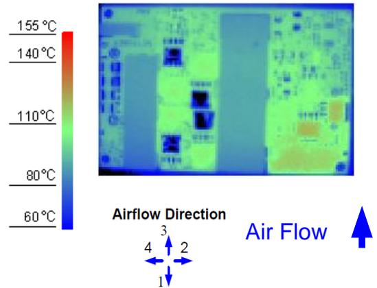
**Figure 10.** Thermal Image for Airflow Direction 3
