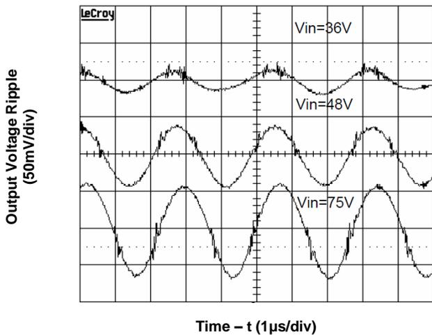
Figure 5. Output Ripple Voltage at Full Load
