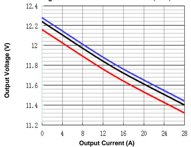
Figure 4. Output Characteristics (parallel option)
