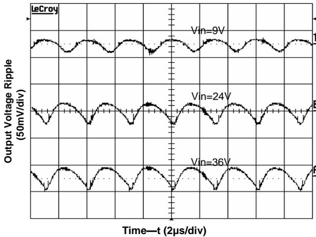
Figure 4. Output Ripple Voltage at 3.3V, 3.5A Output
