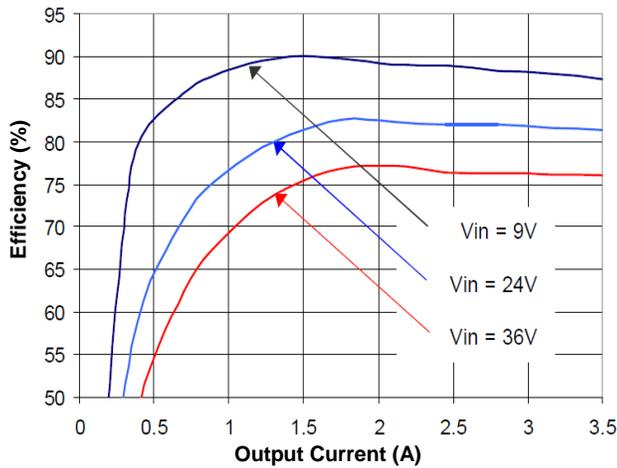
Figure 1(a). Efficiency vs. Load Current (25°C, 3.3V)
