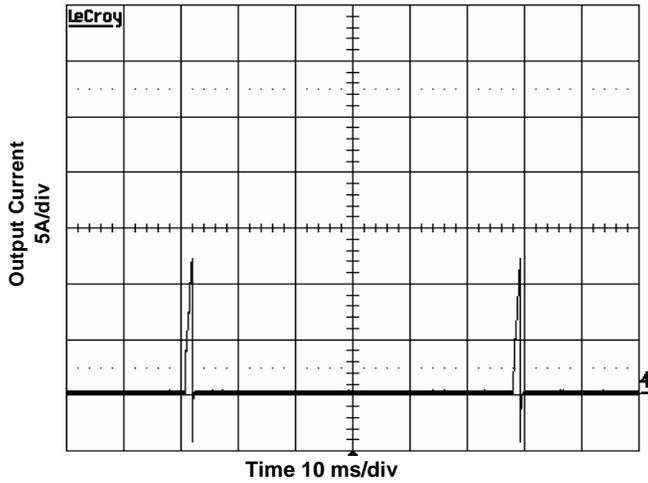
Figure 10. Short Circuit Current. Vin = 24V
