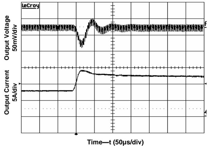
Figure 9. Transient Load Response
