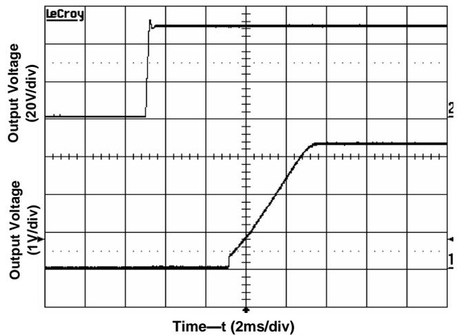
Figure 7. Start-Up from Application of Input Voltage
