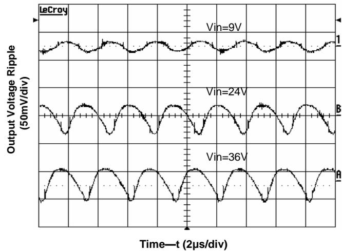
Figure 5. Output Ripple Voltage at 5V, 3.5A Output
