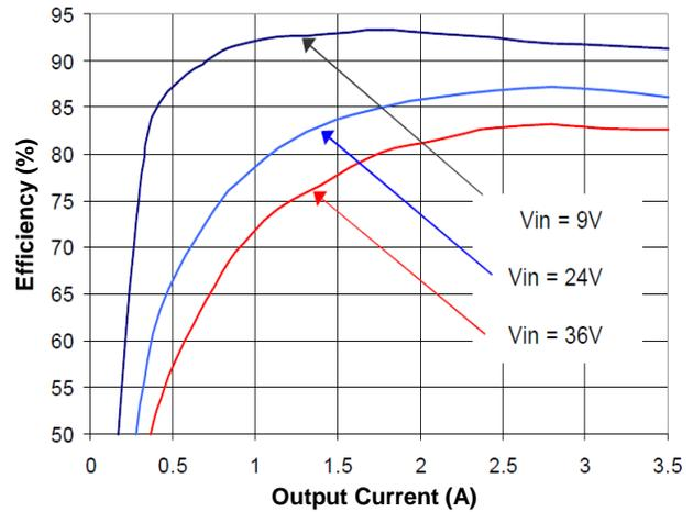
Figure 1(b). Efficiency vs. Load Current (25°C, 5.0V)
