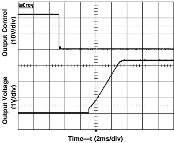
**Figure 4.** Start-Up from Enable Control
