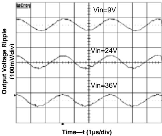
**Figure 6.** Output Ripple Voltage at 5V, 9A Output
