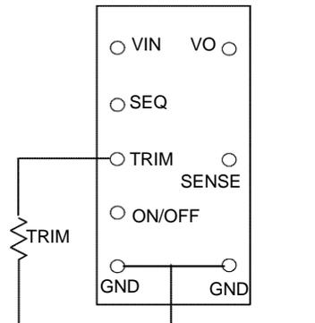
Figure 14. Circuit to Trim Output Voltage.
